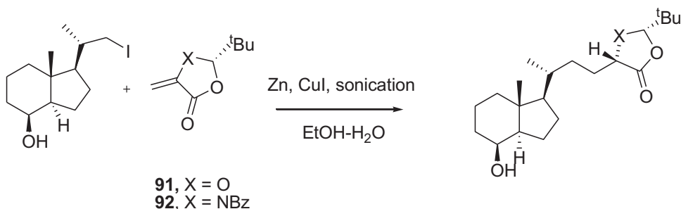
Scheme 47. Zn-mediated RCA on methylene lactones in EtOH–water (Refs. [63–65]).
