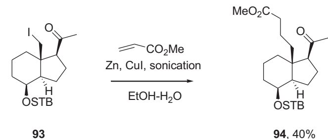
Scheme 48. Zn-induced intermolecular RCA of hindered neopentyl iodide 93 to methyl acrylate (Ref. [66]).
